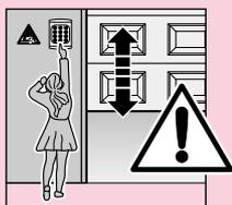
Fixed control units (such as buttons, etc.), must be installed within sight of the door, but removed from moving parts and at a height of at least 1.5 m. It is vital that they are attached out of the reach of children!
