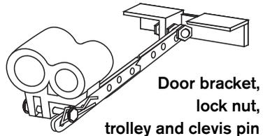
**Door bracket, lock nut, trolley and clevis pin**
