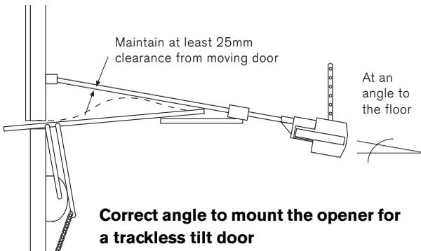
**Correct angle to mount the opener for a trackless tilt door**
