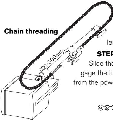
The chain will need to be shortened to suit the choice of pole length and sprocket size.
