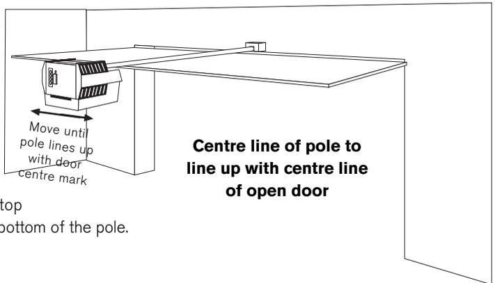
**Centre line of pole to line up with centre line of open door**
