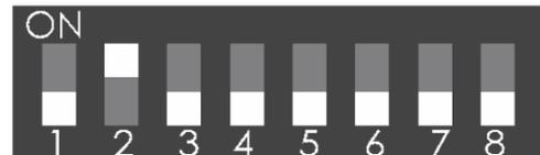
Dipswitches (off on off off off off off off)
