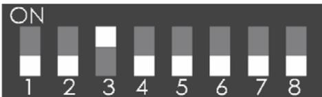
Dipswitches (off off on off off off off off)
